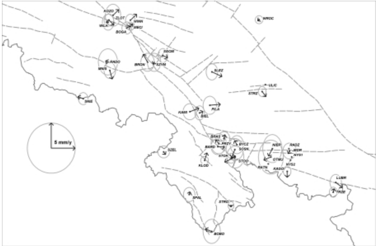
Fig. 5 Horizontal velocities of GEOSUD network points (1996-2004).
